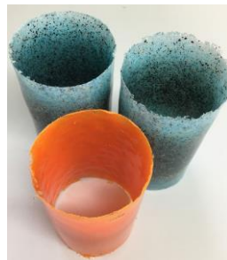
Mould cylinders approximately 95mm Diameter x 150mm Long.
