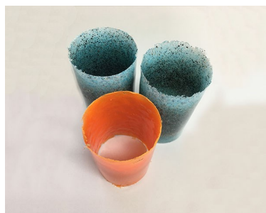
Mould cylinders approximately 80mm Diameter x 140mm Long.
