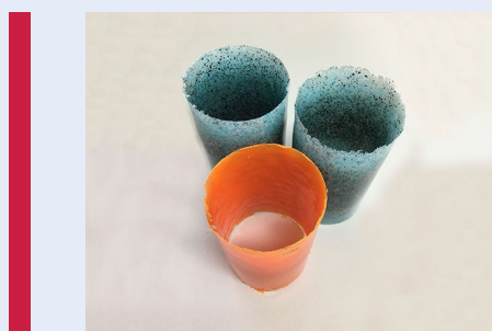
Mould cylinders approximately 95mm Diameter x 150mm Long.
