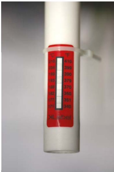
K-Label mounted using a cable tie
