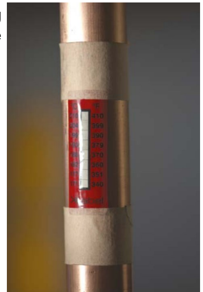
K-Label mounted using adhesive tape
