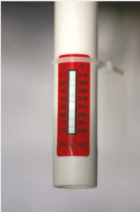
K-LABEL mounted using a cable tie
