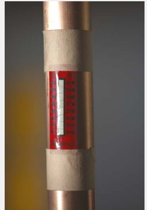
K-LABEL mounted with adhesive tape
